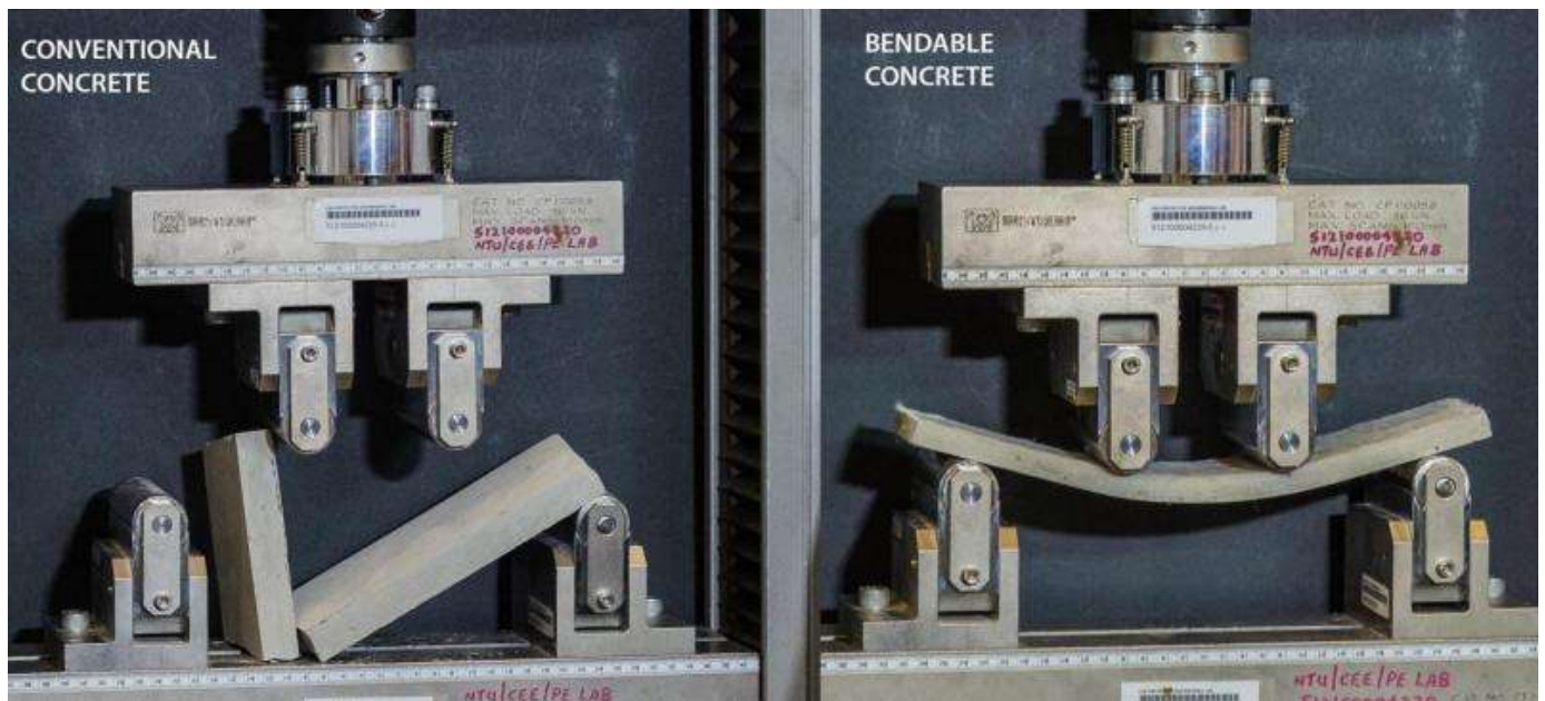
Conventional Concrete vs Bendable Concrete developed at NTU. Credit: Nanyang Technological University
